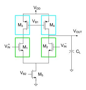
Problem 7 Determine the common-mode input range and the output signal swing of the amplifier you designed in the previous problem.
